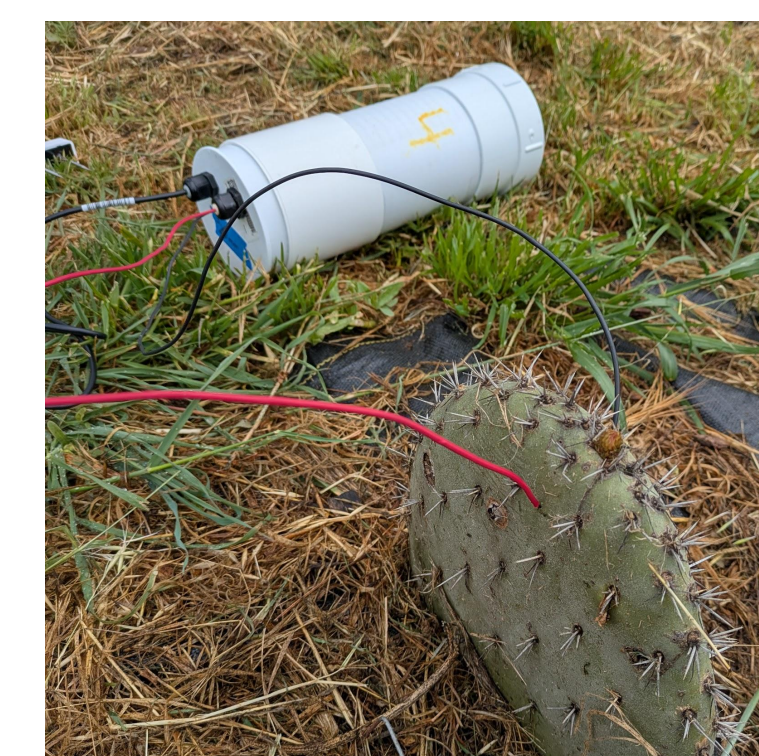
Figure 6: Outdoor deployment of ENTs to monitor prickly pear cacti power output.
