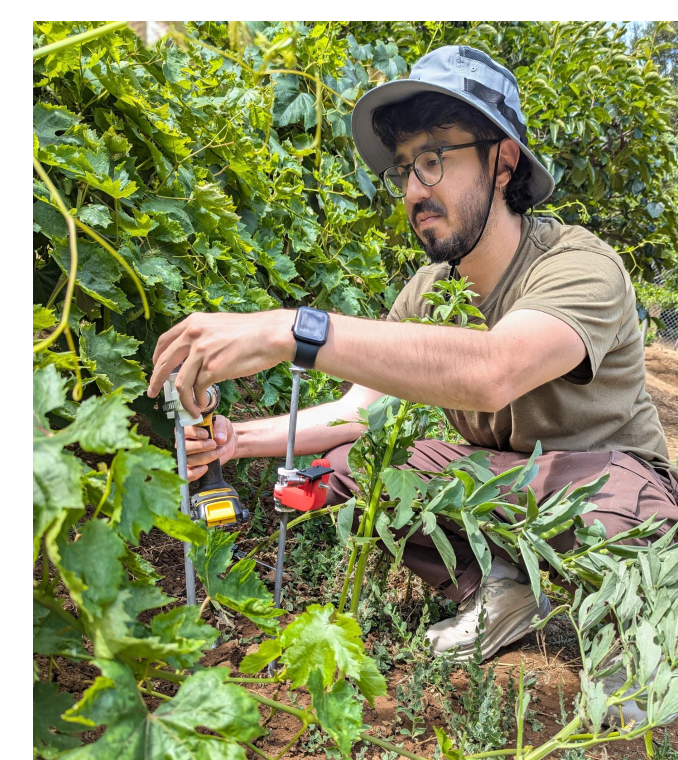
Figure 5: Deploying bio-mimetic leaf wetness sensor in the field
